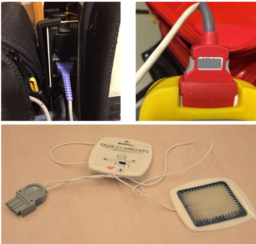
Figure 9. Specific details that users brought to the WS. Above left: a perceived bad example of connectors. Above right: a perceived good example of connectors. Bottom: electrode pads, representing a good design to teach positioning of electrodes on the body.
