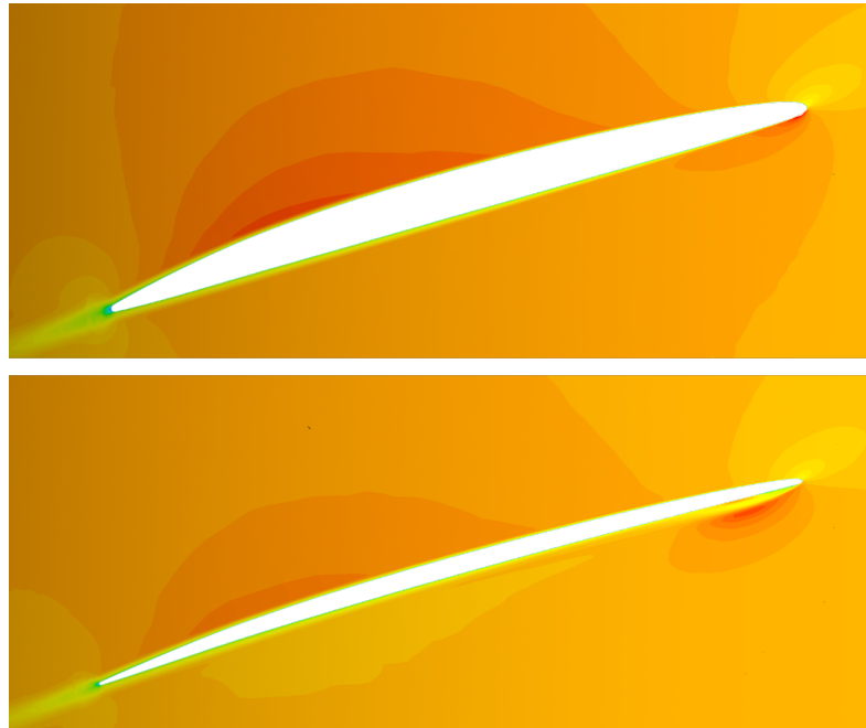
Figure 9: Ship-Scale CFD results; contours of velocity magnitude in a reference frame rotating with the propeller at a radial section at r/R = 0.9 . Ice classed propeller (top) and conventional propeller (bottom). Contour scale 0-23 m/s.
