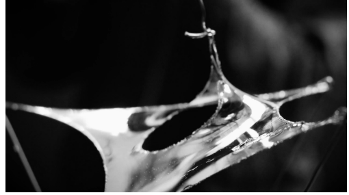
(c) A 'Frei Otto eye' form-found using soap film and cotton threads
