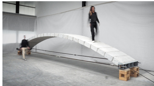
(b) Bridge made of re-used concrete (2021)
