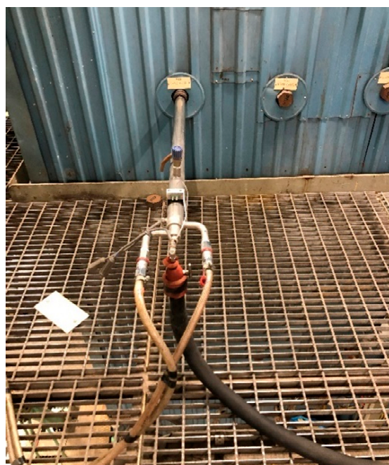
Figure 12. Flue gas sampling probe applied in the measurements performed over the cross-section of the combustor.
