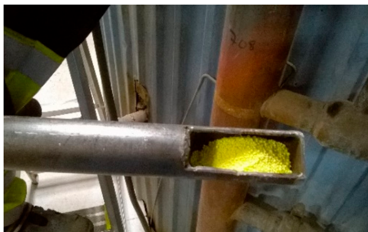
Figure 11. Batch probe for addition of sulfur granulates to the flue gas stream leaving the cyclone.
