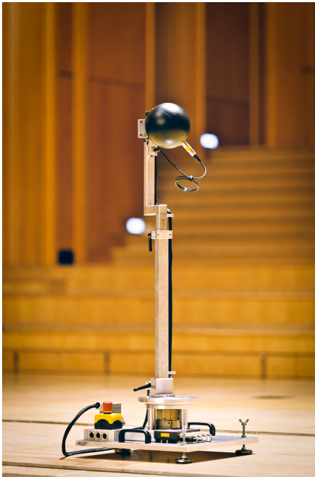
Figure 1.4: VariSphear SMA measurement device to capture ARIR data [5]. Image from [12] licensed under CC BY 4.0.
