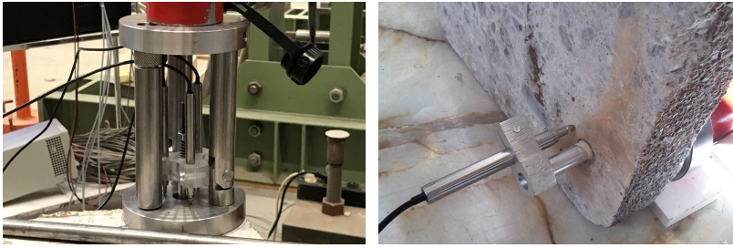
Figure 3.9: Photographs of pull-out rig and slip measurement devices. Note that specimen to the right is tilted with respect to normal testing position to better show the measurement device.
