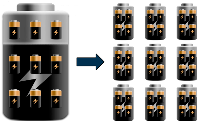
Figure 3.1: Rearrangement of the high voltage battery pack into a modular battery system consisting of small, generic battery packs.
