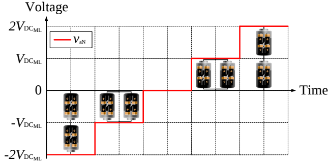
Figure 3.11: Possible phase output voltage levels and battery module configurations for a CDHB inverter with two SMs per phase, n = 2 .
