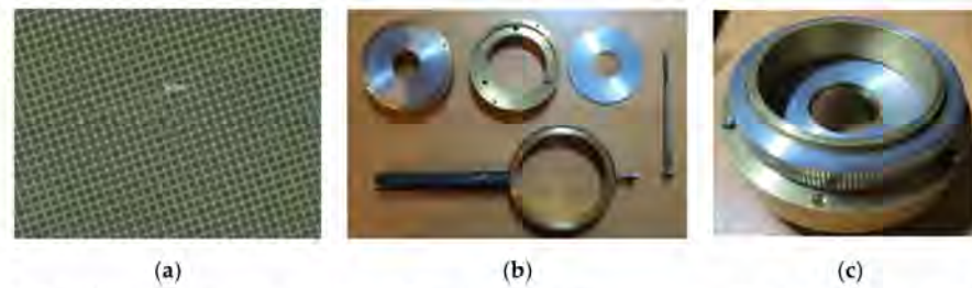
Figure 10. Tunable interferometer: (a) golden mesh evaporated on quartz substrate; (b) mechanical parts of the gadget; and (c) assembled interferometer.
