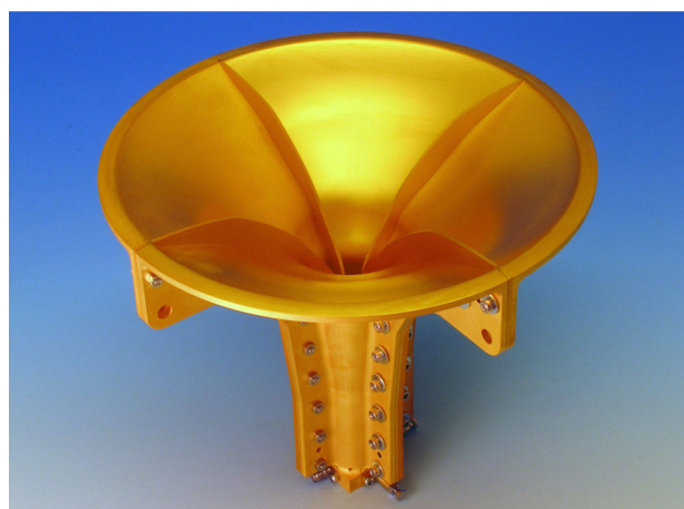
Fig. 8 The wideband feed horn used to simulate ground-noise pickup when mounted in one of the VGOS antennas at Onsala
