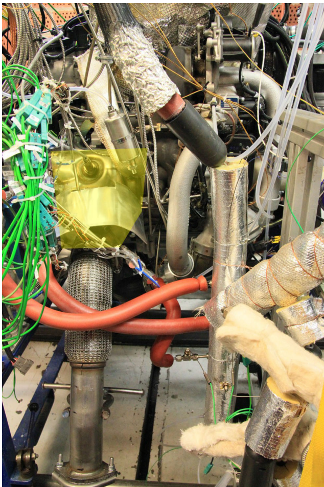
Fig. 8 The experimental setup, with the TWC housing and heat shield highlighted. The turbocharger is just visible to the right of the TWC. The exhaust from the TWC is fed down through the visible ducting
