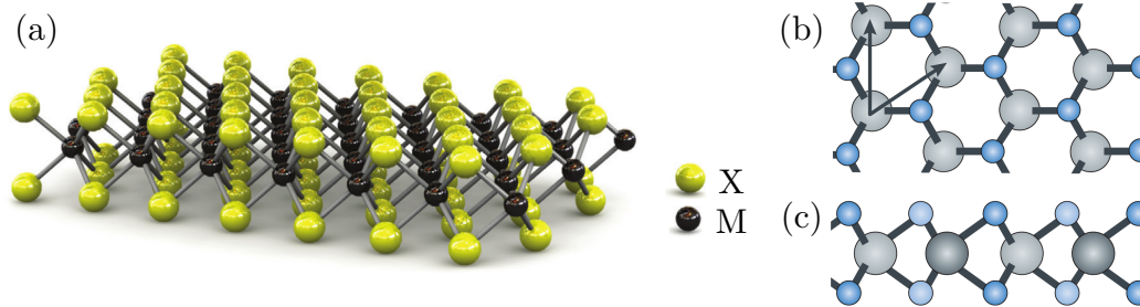
Figure 1.1: (a) Three-dimensional representation of the atomic structure of a TMD monolayer. (b) Top and (c) side perspectives of a TMD monolayer. The arrows represent the lattice vectors. Figures taken from (a) Ref. [12] and (b) Ref. [13].
