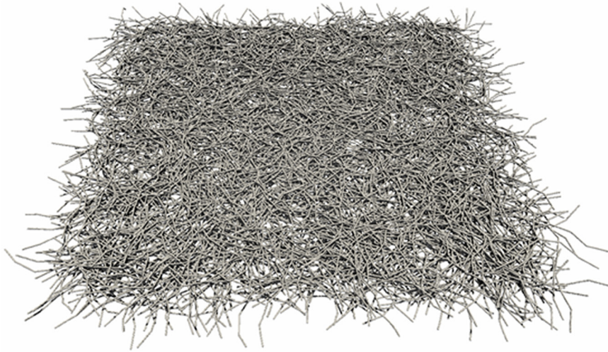
Fig. 4. Illustration of fibre network used in the simulations. The network consists of 3000 fibres with a length of 2 mm deposited in a 1x1cm area.
