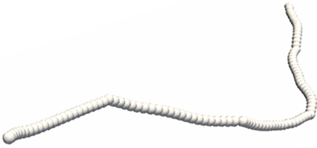
Fig. 2. Illustration of a fibre modelled as a string of 110 connected particles.
