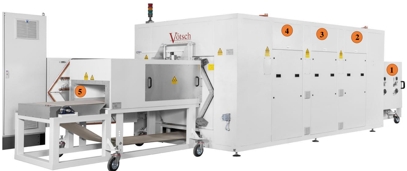
Figure 1. A side view of the HEPHAISTOS microwave oven system. Main modules of the oven are represented by number tags 1, 2, 3, 4, 5. Tag 1 and Tag 5 represent the entrance of the wet foam and exit doors for the dry foam, respectively on the conveyor belt. Tags 2, 3, 4 indicate the three modular heating system with inbuilt hexagonal cavity with high power microwave heating sources and control system block. The MWT system will be integrated near the entrance door. The system is located at KIT, Germany.
