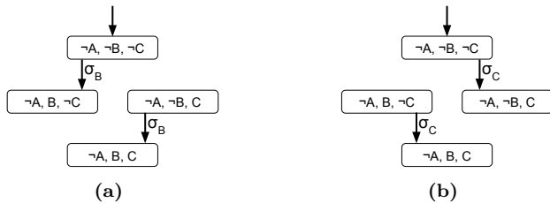
Figure 3.5: The modular model so far after Step 3.2, with module L_1 in (a) and module L_2 in (b).
