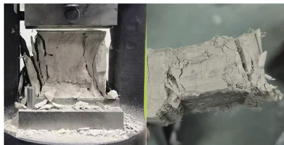
(b) Comparison of the failure patterns of LC3-ECC specimens with and without PP fibers
