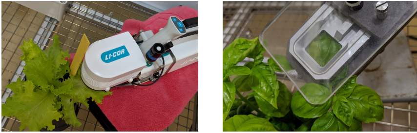
Figure 3.2: An infrared gas analyser, for measuring the photosynthetic rate in terms of \text{CO}_2 uptake per \text{m}^2 leaf area and s. Mounted with a leaf cuvette combined with a light source (left), and a clear leaf cuvette allowing the ambient light reaching the leaf (right).
