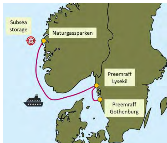
Figure 1: Location of the Lysekil and Gothenburg refineries, the onshore terminal at Naturgassparken in Øygarden and final sub-sea storage in the Norwegian Continental Shelf. The Preem CCS project considers ship transportation of liquefied CO 2 .
