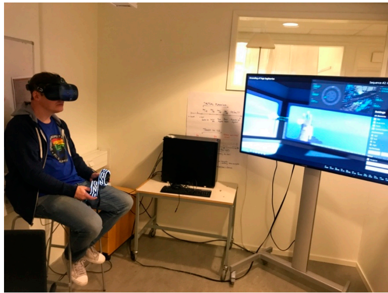
Figure 3. VR/AR test setup at Chalmers University, showing one of the users wearing the VR headset and using portable controllers to interact and move around on the virtual ship bridge.
