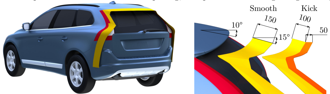
(a) Rear view of the Volvo XC60 with a tapered 3/4 cavity.
