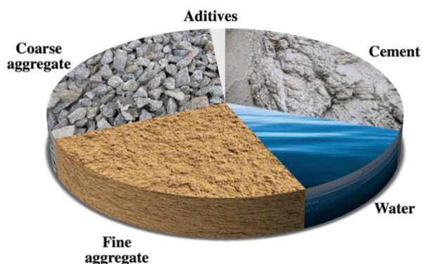
Figure 1. Diagram of standard concrete composition
