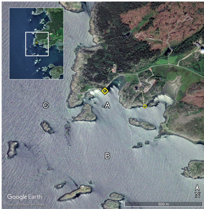
Fig. 13. Demonstration of the impact of wind direction and the complex coastlines on the SSR over different areas nearby the Onsala GNSS-R station. The station is shown by a yellow diamond symbol.
