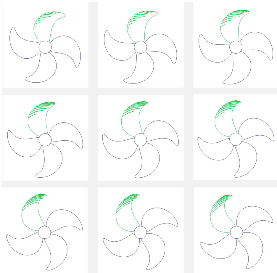
Figure 5. Cavity shape on blade in 9 time steps.
