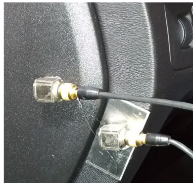
Figure 10: Two triaxial piezoelectric accelerometers located on the cockpit left cover to measure the relative motion between the two parts.
