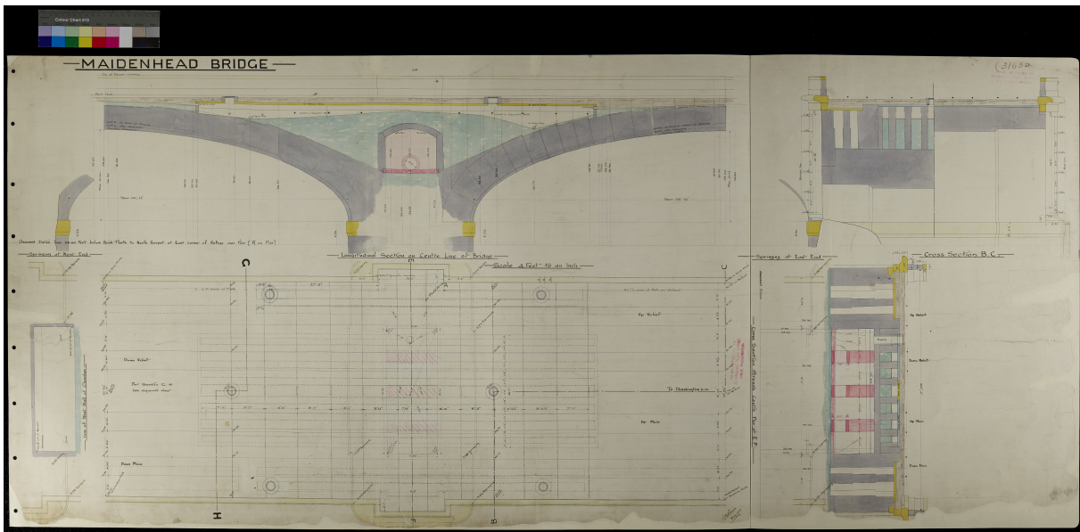
Figure 2: Cross section through chamber of Maidenhead Railway Bridge, image from Network Rail Corporate Archive
