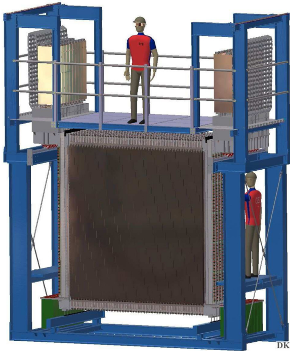
Fig. 11. Schematic layout of one NeuLAND frame supporting 15 double-planes in total, here equipped with 12 double-planes. A maintenance platform on top of the double-planes allows for easy access to the readout electronics hosted in the boxes on both sides above of the double-plane, the high voltage supply boards are located in the lower left and right corners of each double-plane.
