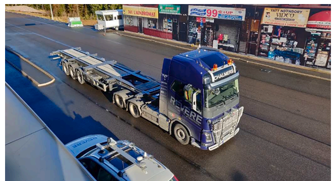
Fig. 3. Volvo FH tractor semi-trailer combination used in the experiment. All pictures and videos (except Fig. 6) have been taken either during the pilot test or after the experiment, and are reported here to support the readability of the paper. To avoid interfering with the experiment, none of these recordings were done during the actual data collection. The setup during the experiment might therefore differ slightly from the one shown in the images/videos. In particular, the white tent used to hide the stationary dummy was not present during the recordings.
