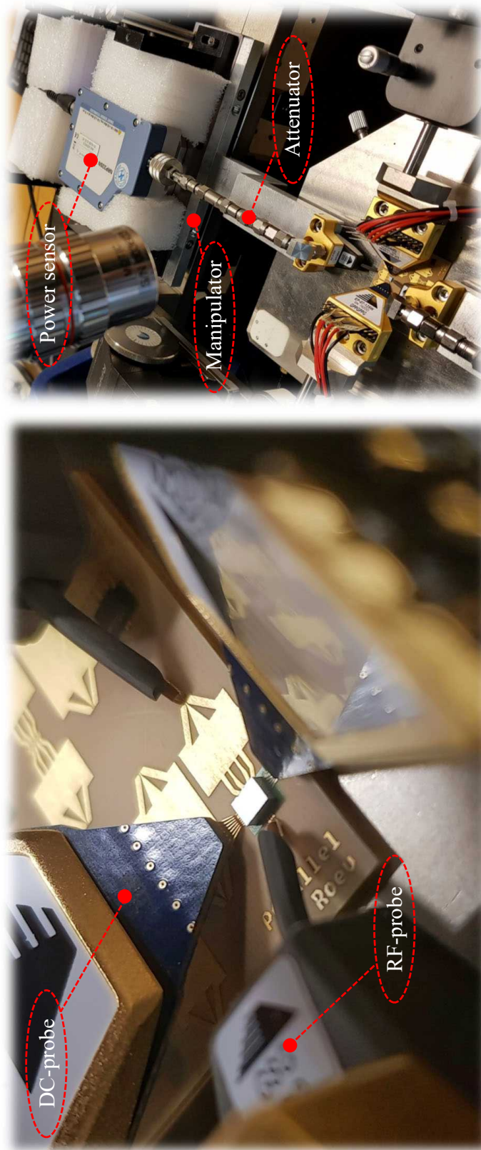
Figure 4.27: Photo of the measurement setup. The measurements are carried out using a Cascade Microtech mechanical probe station with four manipulators.
