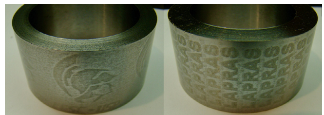
Fig. 26. Examples of grinding-imprinted patterns [21].
