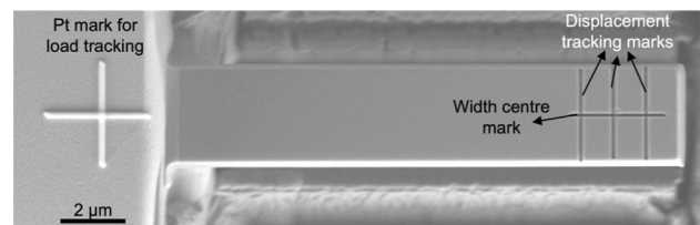
Fig. 1 Top view of a FIB milled microcantilever used for cyclic bending showing a platinum marker used for measuring load, and FIB-milled markers towards the free end used for tracking displacements
