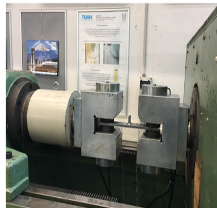
Fig. 3. L: Schematic figure shows the hydraulic clamp. R: Fatigue testing rig.
