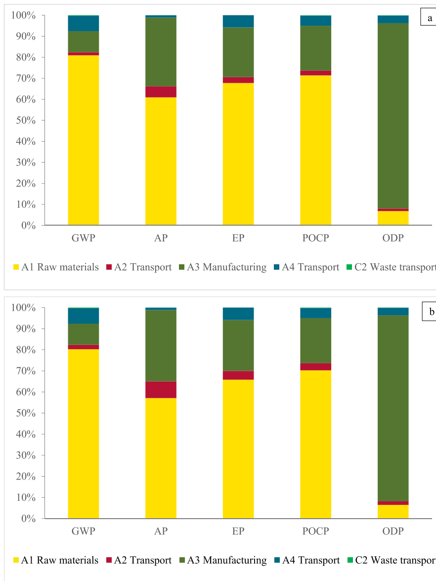
Fig. 12. Distribution of environmental impact categories over the life cycle phases for: a) cement composite with wood residues; b) cement composite with tyre fibres. GWP - global warming potential, AP - acidification potential, EP - eutrophication potential, POCP - photochemical ozone creation potential, ODP - ozone depletion potential.
