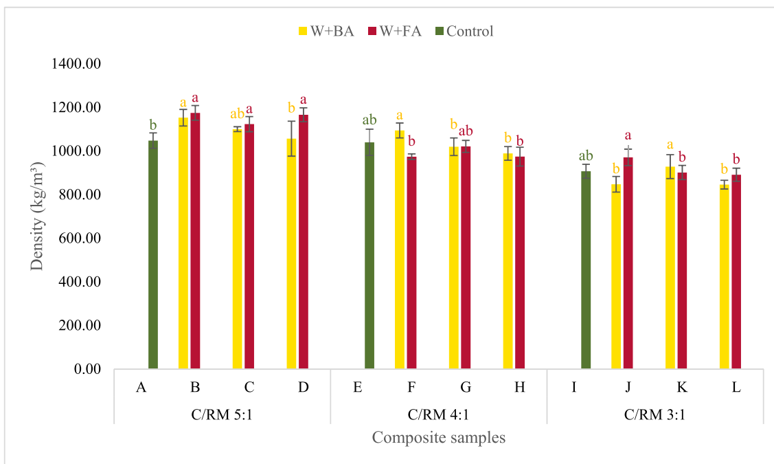
Fig. 3. Density of cement-bonded composites with wood residues. [Error bars represent standard deviations of three replicates. Within each C/RM ratio group, columns with the same letter (a, b, ab) are not significantly different (significance level \alpha = 0.05 )].
