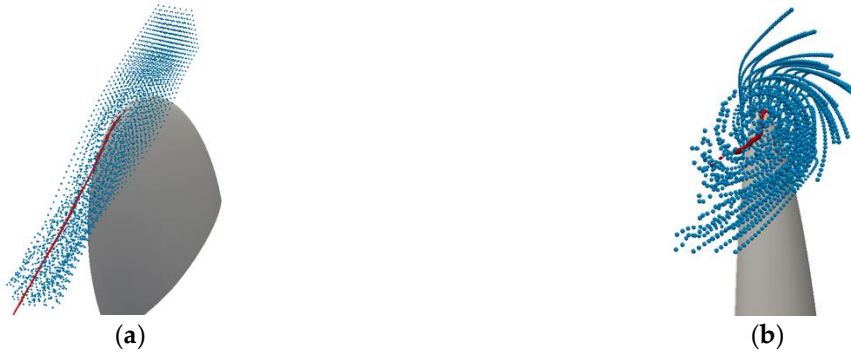
Figure 3. Nuclei transport towards the vortex core: (a) top view (b) front view. The bubble nuclei are enlarged by 150R and the red line depicts the vortex central line. The nuclei have initial diameter of 5 \mu\text{m} .
