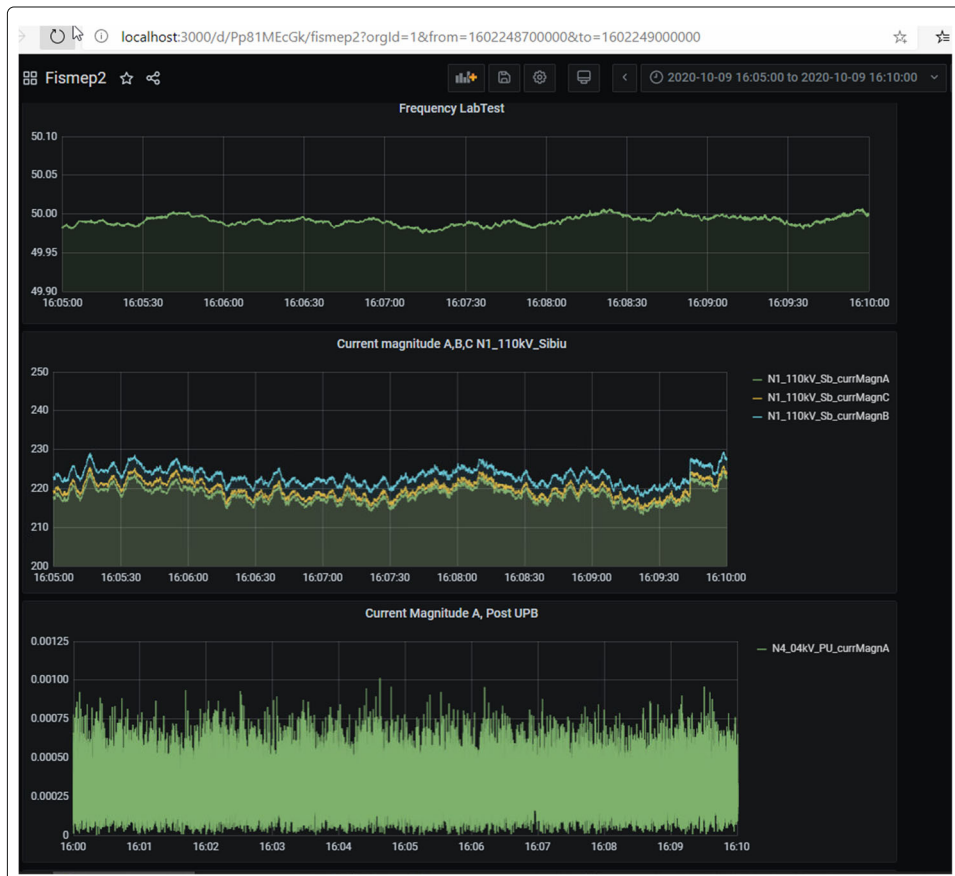
Fig. 12 Monitoring of the currents and frequency in Power Grid using software application
