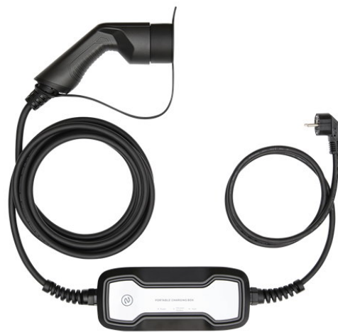
Figure 2. Single-phase charging cable with Schuko and Type 2 connector including in-line integrated EVSE to adjust the charging current reference between 10 A and 16 A from Deltaco [29].
