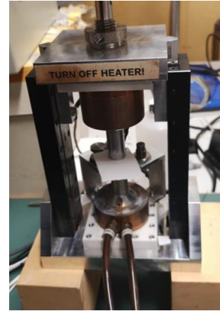
Fig. 2 Steady state heat-flow setup for through-plane thermal conductivity measurement.
