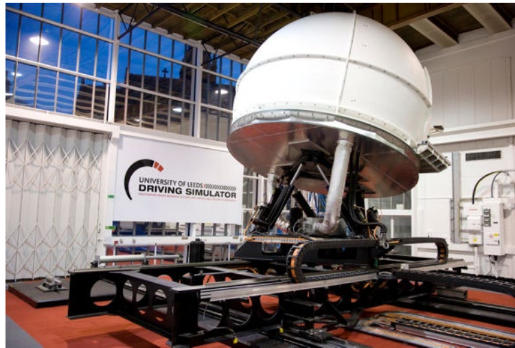
Figure 4 One of the most technically advanced motion-base high-fidelity simulator in the world today, available at the University of Leeds
