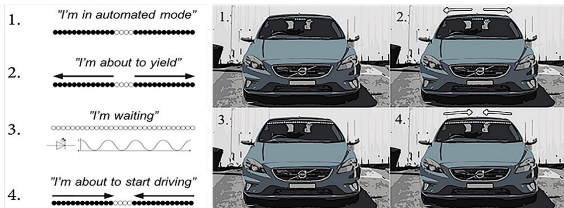
Figure 7 - Automated Vehicle Interaction Prototype (AVIP) signals for communication of intent and automation mode to pedestrians (Habibovic et al., 2018).
