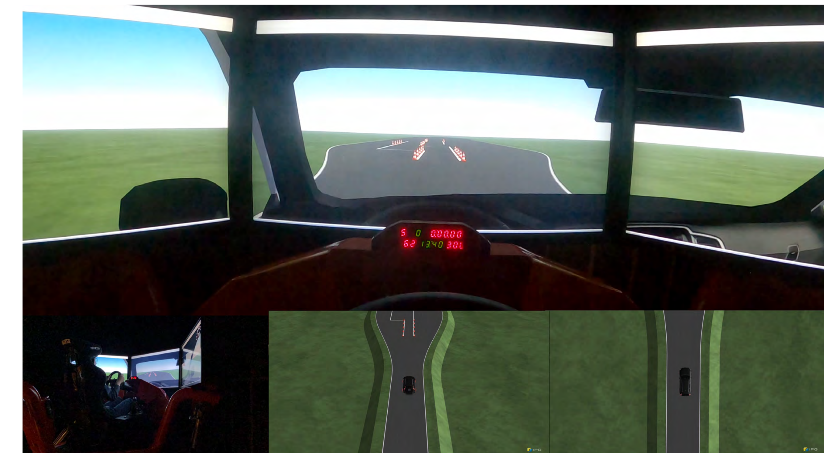
A DLC test with motion simulator
