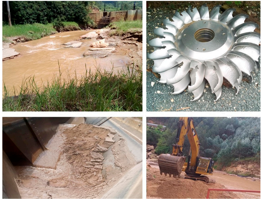
Figure 3. Field observation on soil erosion, sediments, and turbine wear. Clockwise from upper left: an upstream catchment filled with sediments and soil erosion during one rainy season, turbine runner wear due to waterborne sediment after 1.5 years in operation, heavy equipment removing sediments from another upstream catchment, and a sediment basin filled by sediments over three days during rainy season.
