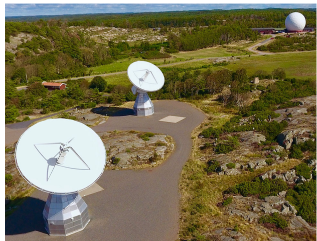
Fig. 1 The Onsala telescope cluster used in these observations: OW (left), OE (middle), and ON (right; inside radome). OW and OE are about 75 m apart, and the baseline between ON and OE is about 470 m long. Credit: Onsala Space Observatory/Roger Hammargren
