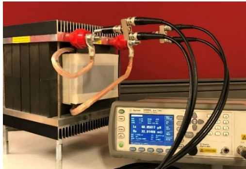
FIGURE 17. The test setup for leakage inductance measurement.
