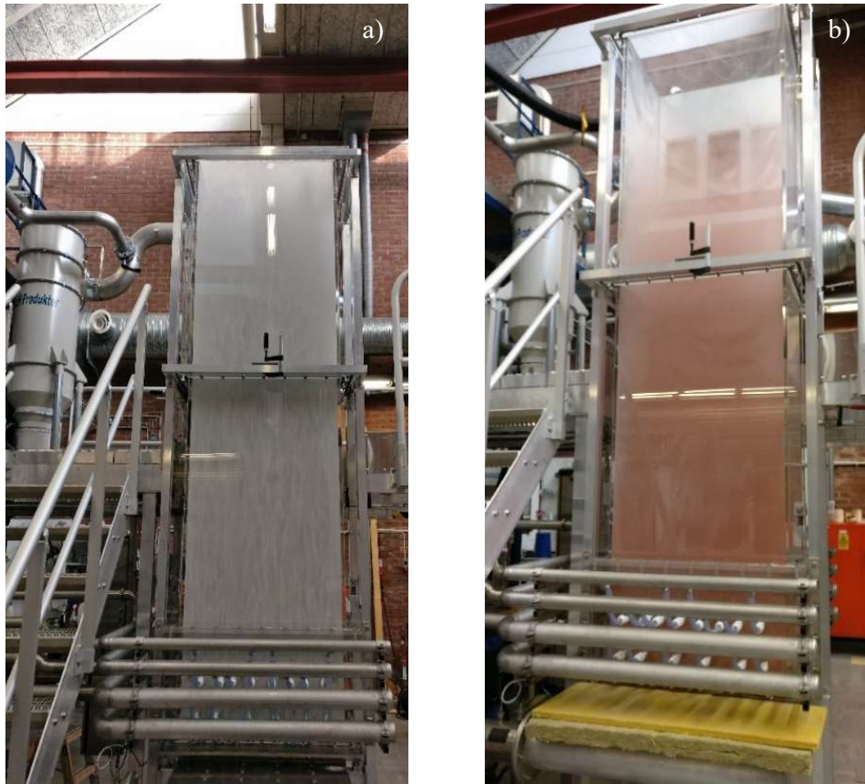
Figure 8. Photographs of the cold-scale model with: a) non-scaled particles (glass particles); and b) scaled particles (copper).
