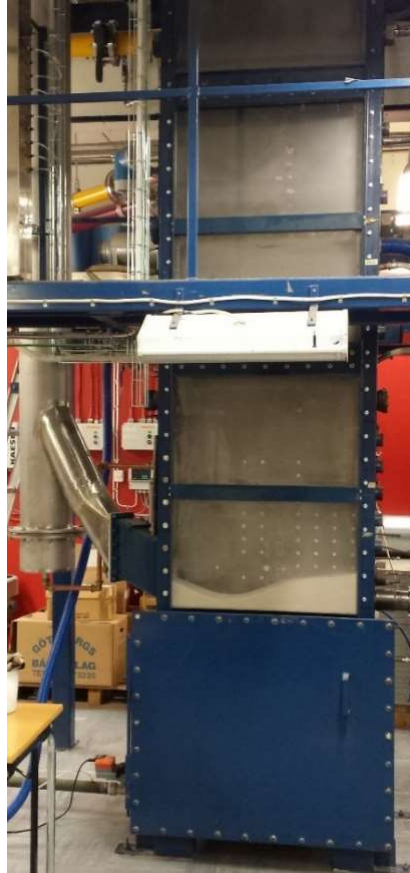
Figure 5. Bottom part of the pseudo-2D unit.
