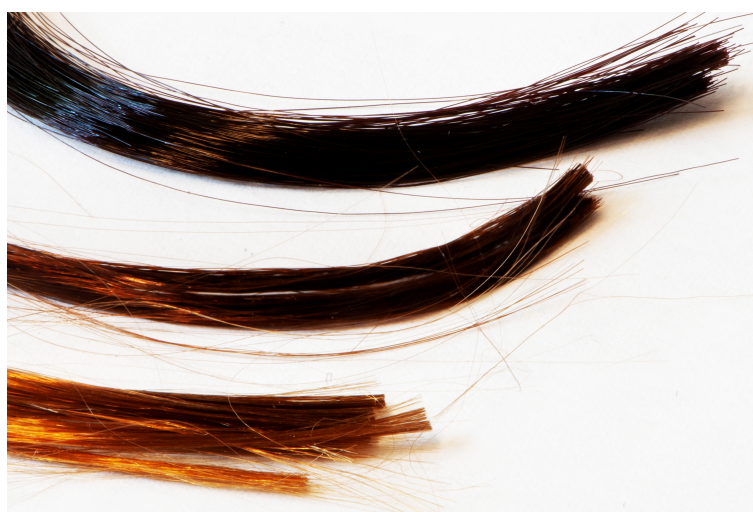
Figure 23. Photography of three cellulose-lignin fibers containing different amounts of lignin. Top: 67, Mid: 33, Bot: 10 wt% lignin.
