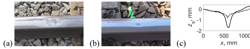
Fig. 6. Photograph of severe squat A (a) and light squat B (b) at shunting yard Munich North. Corresponding squat profiles at midline (c): — squat A, -.-. squat B.
