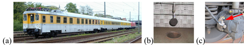
Fig. 1. Noise measurement car of DB Systemtechnik (a) equipped with a microphone above the measurement bogie (b) and accelerometers on the axle boxes of the measurement bogie (c).
