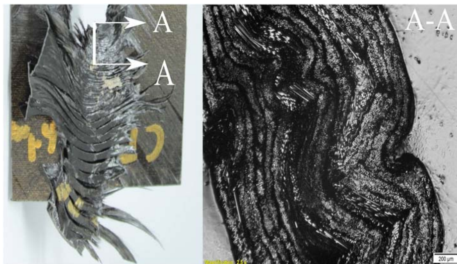
Figure 17. Deformation of the material around the bolt post tearing test.
