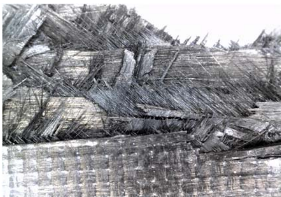
Figure 8. Fracture surface of CF-PP TBDC tensile specimen.
