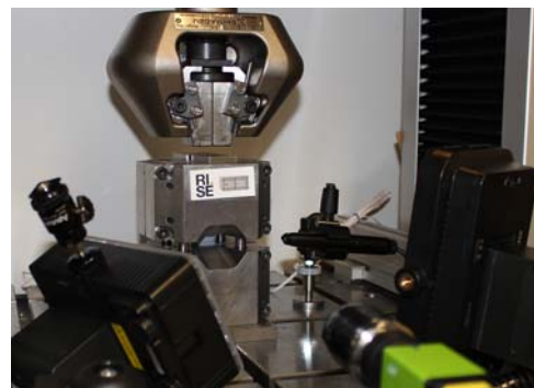
Figure 4. Compression test setup with DIC system and modified CLC fixture.
