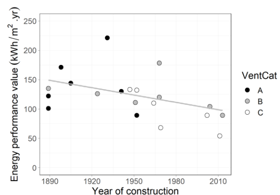
Figure 2. Energy performance value against year of construction of the buildings. Regression line is added for the whole sample. VentCat: Ventilation category.
