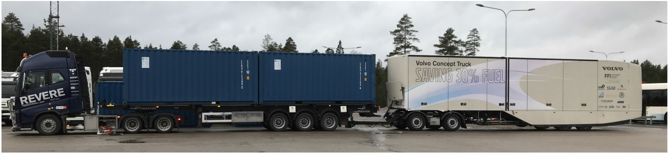
FIGURE 6. A-double long combination vehicle used for collecting experimental data.
