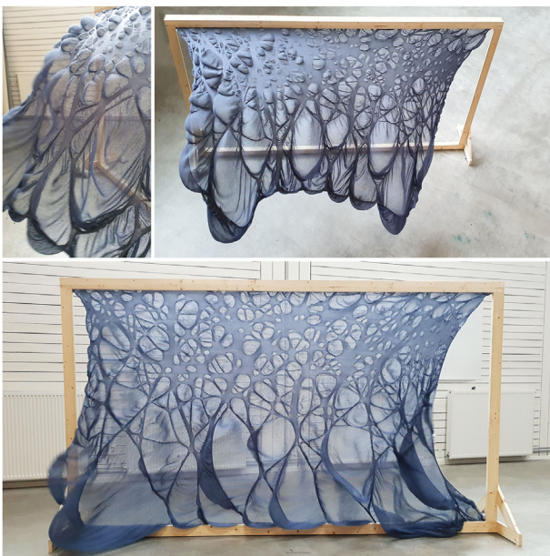
Fig. 23 Wind studies of the drop-stitch textile mounted on a wooden frame. Top: textile only fixed at the top. Bottom: textile attached to both top and bottom of the frame.
