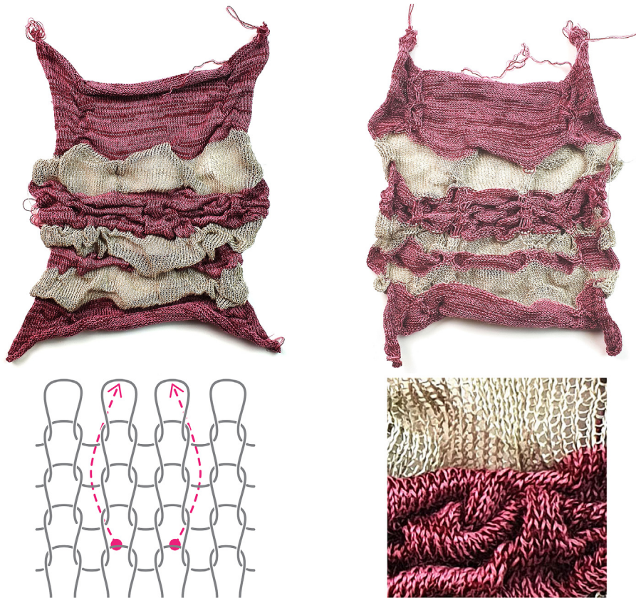
Fig. 12 Top: sample produced using the hanging stitches technique, seen from the right, and purl side. Yarns: wool 28/2 × 3 in two shades of pink, stitch length 5, and uncoloured linen, stitch length 7. Knitted on 80 needles. Bottom: illustration of the knitting technique and a close-up. Note, this sample was fixed at a set of points to keep edges from curling in.
