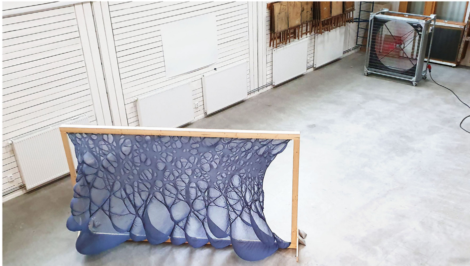
Fig. 7 Wind-machine set-up for the larger drop-stitch sample described in Section 4.4.
