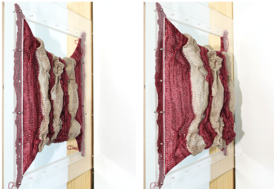
Fig. 13 Hanging-stitches knit. Left: in relaxed state. Right: exposed to airflow (Note: mounted with the knitting direction from left to right).
