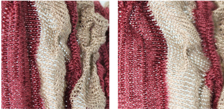
Fig. 14 Hanging-stitches knit, close-up. Left: in relaxed state. Right: exposed to airflow.
