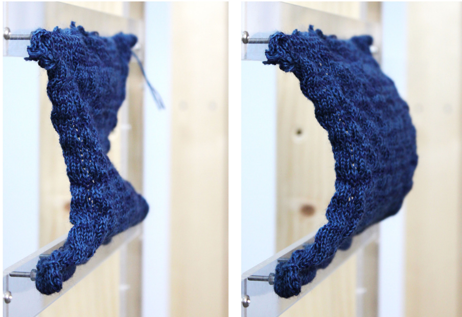
Fig. 10 Tuck-knit. Left: before airflow was applied. Right: exposed to airflow.
