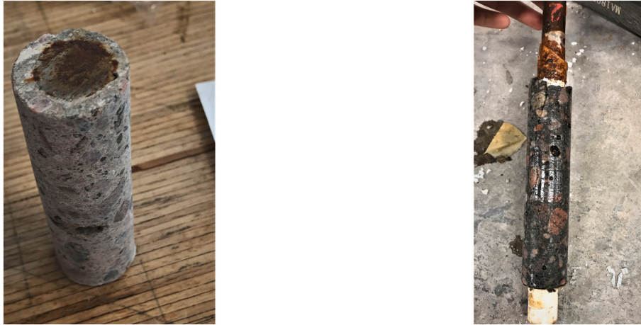
Fig. 2. Samples included in the study, after coring. To the left, naturally corroded sample cored from a decommissioned bridge; to the right, artificially corroded sample with corrosion induced cracks.
