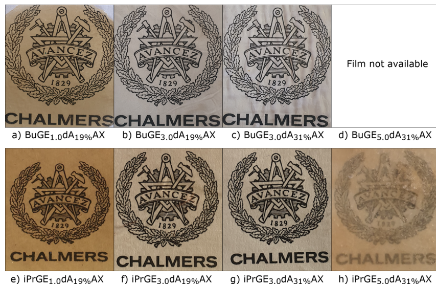
Figure 4. Films fabricated from the activated AX ethers using BuGE (a–d) and iPrGE (e–h) via compression molding at 140 °C and 50 kPa pressure. The Chalmers logo is used to determine the transparency of the films. Chalmers University of Technology gave permission to use and does not claim any copyrights. BuGE 5,0 dA 31% AX film (d) is not available because the material was too soft to form a free-standing film.
